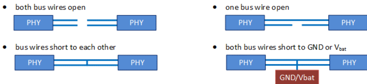
Figure 1 Overview of error situations to be detected.
