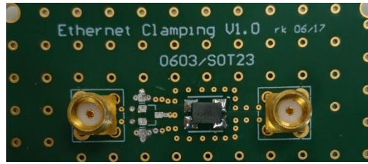
Figure 5-12: Example of RF clamping test board for ESD suppression device, top layer
