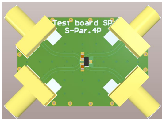
Figure 5-5: Example of test board 4-port S-parameter measurement for ESD suppression device, top layer
