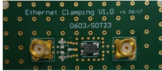
Figure 5-12: Example of RF clamping test board for ESD suppression device, top layer
