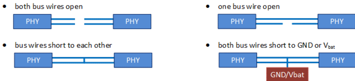
Figure 1 Overview of error situations to be detected.
