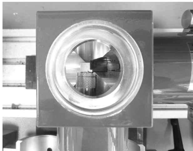
Figure 87: Connector coupling and screening attenuation measurement setup example for right angled PCB connectors
